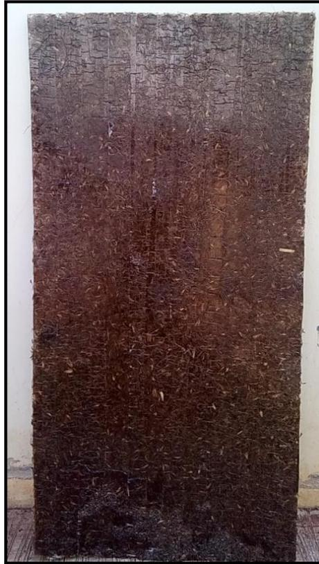
Gambar 1 *Fiber Roof Building* Berukuran 100 cm x 50 cm x 6 mm
