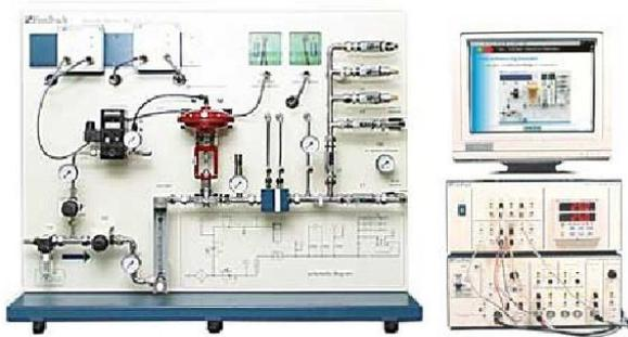
Gambar 1. *Pressure Process Rig*
