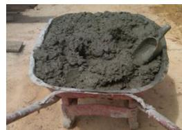
**Gambar 6. Sampel Beton**
